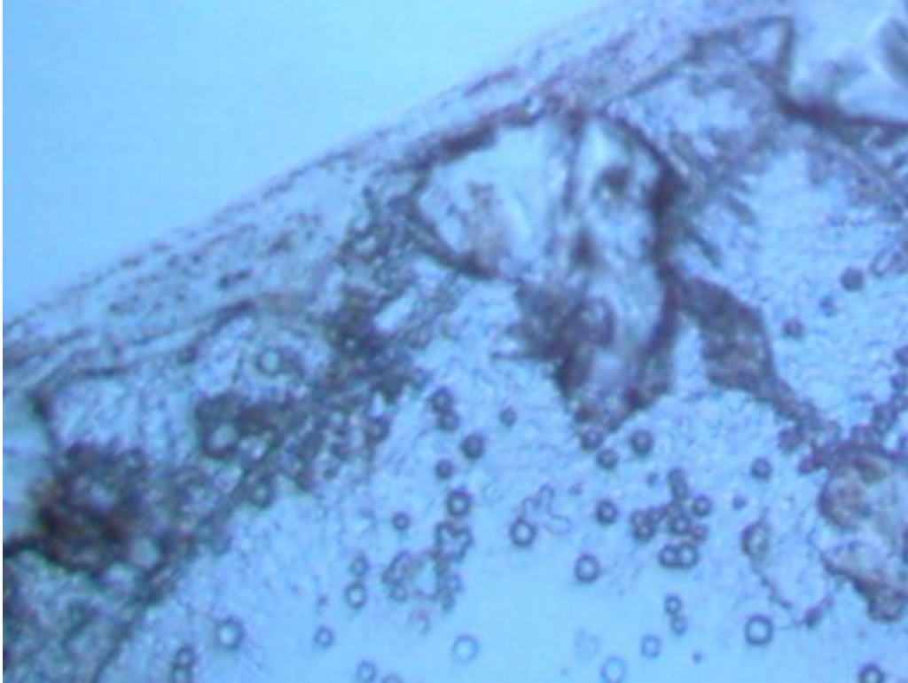
Evaporated Crystal Form; Magnification Approx. 500x Combination of spherical bodies and large crystal formation. Occurs near perimeter of evaporated crystal.
