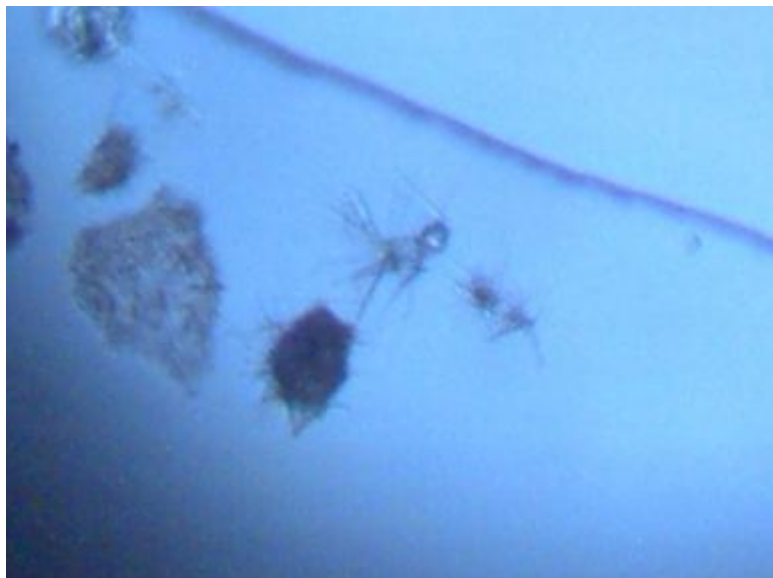
White powder subjected to sulfuric acid 480x Crystal formations apparent
