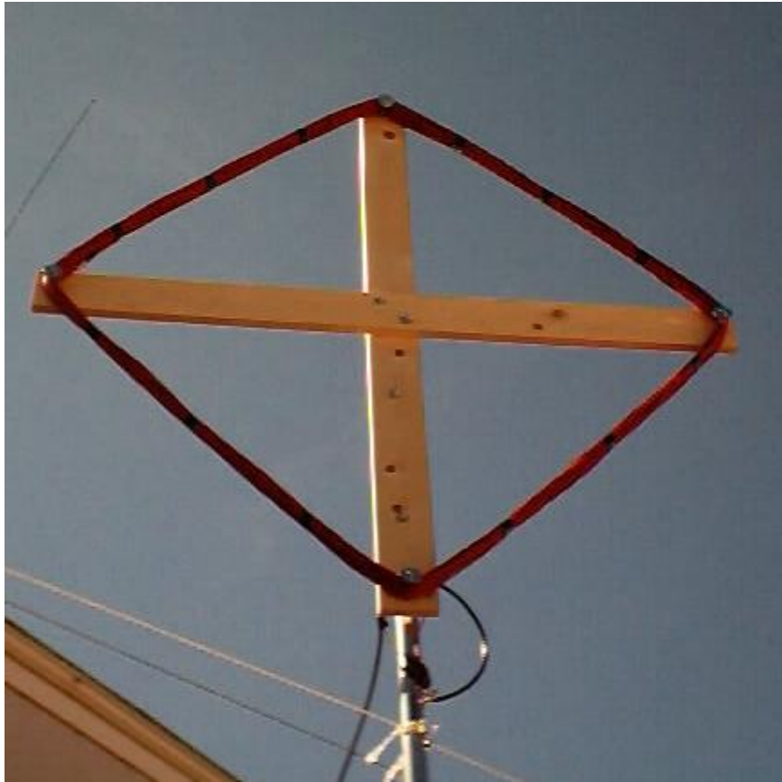
View of Loop Antenna from the ground.
