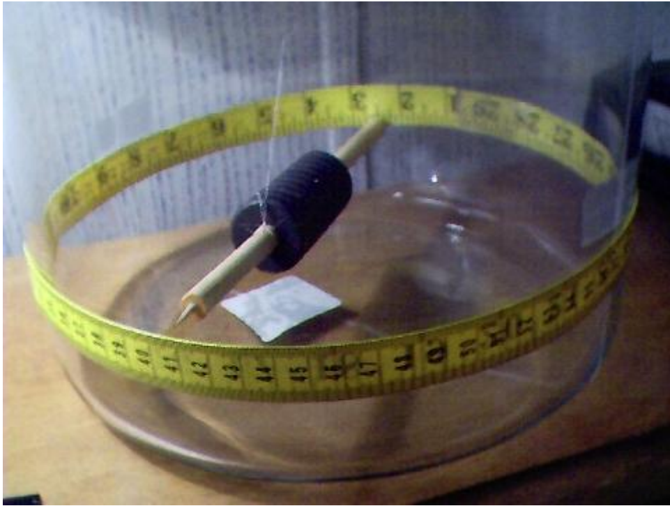
Photograph of the suspended dowel, pointer unit, dowel, magnets and graduated scale.
