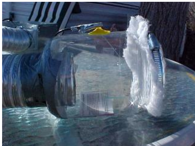
Another view of the container used, with the electrode visible. Porous filter material attached with a hose clamp reduces the flow rate and contains the atmospheric gas subject to the electric field.
