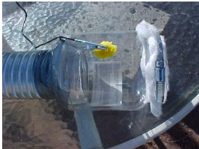
The plastic collection container with electrode and 2 internal glass microscope slides
