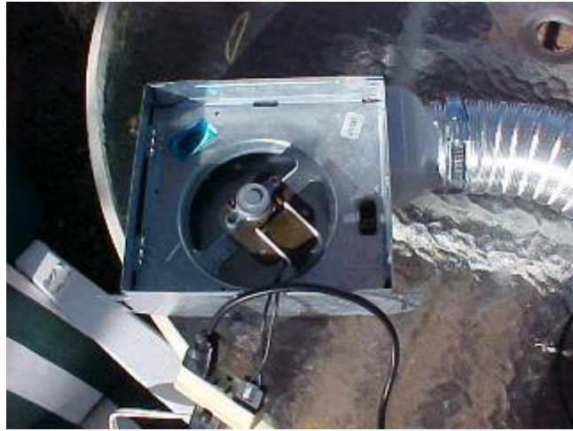
The electric ventilator fan with duct hose attached
