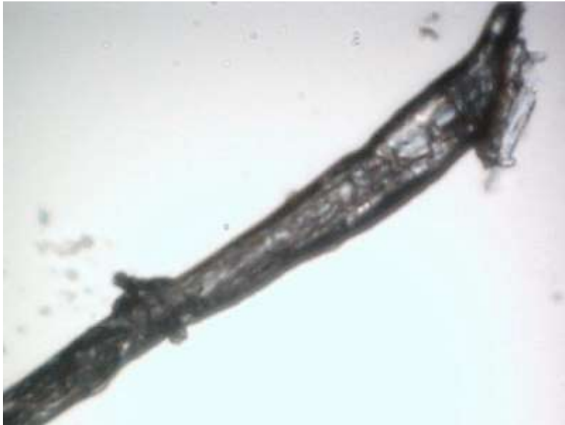
Magnification approximately 1400x. Note variation in fiber form and internal structure becoming evident. Notice irregularities on the surface of the fiber. Notice translucent quality of the fiber.
