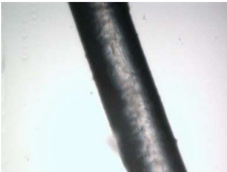
Human Hair : FOR CONTROL PURPOSES ONLY Magnification approximately 700x.. Note smooth outline and uniform size. Measurement : approximately 65 microns across. No significant internal structure or form apparent.
