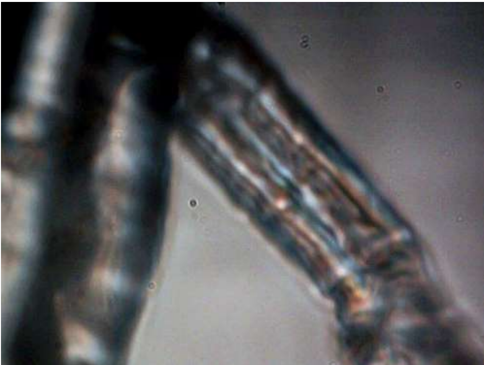
Magnification approximately 5600x. This photograph shows the ability of the fiber to be folded and/or twisted. Internal parallel organization of sub-fibers is visible. Non-uniformity of the fibers dimensions is also evident. Transverse separation or structure also visible in lower right of image.
